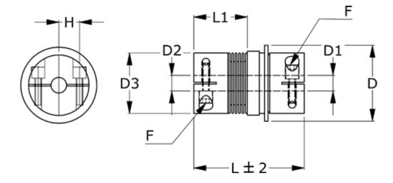
D = 109Nom. torque NM (Tkn) = 200NM overload torque range 2 D1 = 40Position engagement = C = Synchronous
